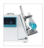
Tilt angle adjustment from 0 to 20° for maximum mixing efficiency.
